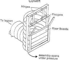
Culverts like this one allow for mosquito control during the Summer months when the gates are closed. During the winter the gate is opened allowing the marsh to act as the filter, base of the food chain, and nursery for the IRL.
