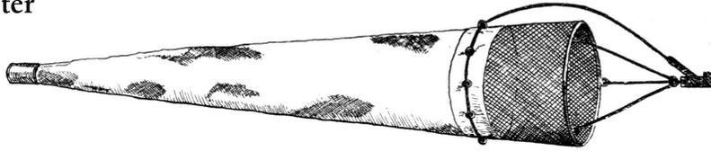
Plankton is caught with a plankton net. The net is made from a very fine mesh nylon or silk cloth. The end of the net is a bottle to trap the plankton inside. Plankton nets can be set out in an area with a strong current, or the net can be pulled behind a boat. Plankton samples can be preserved in 3-5% formalin solution.
